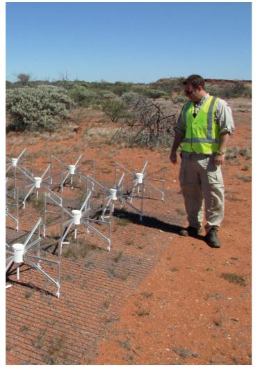
The Murchison Widefield Array telescope at the MRO.
